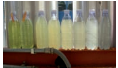
Monitoring during purging as the iron in solution (green) passes to clear water
