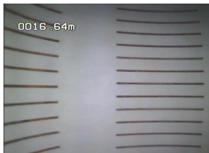
A downhole camera survey shows before (left) and after treatment (right) with BoreSaver Ultra C PRO
