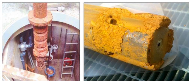
Iron-related deposits on well pumping equipment
