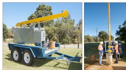
Well rehabilitation rig used in BoreSaver maintenance programmes
