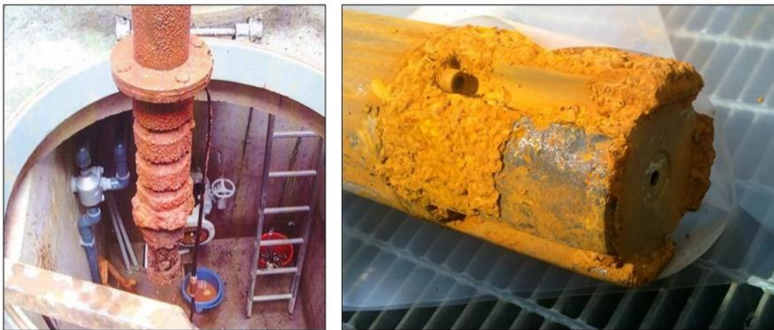
Figure 1. Iron deposits in wells and pumps
