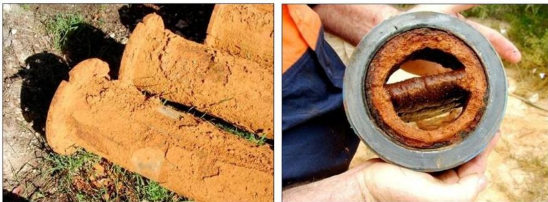
Figure 7. Iron contamination of pipework and valves on mine site
