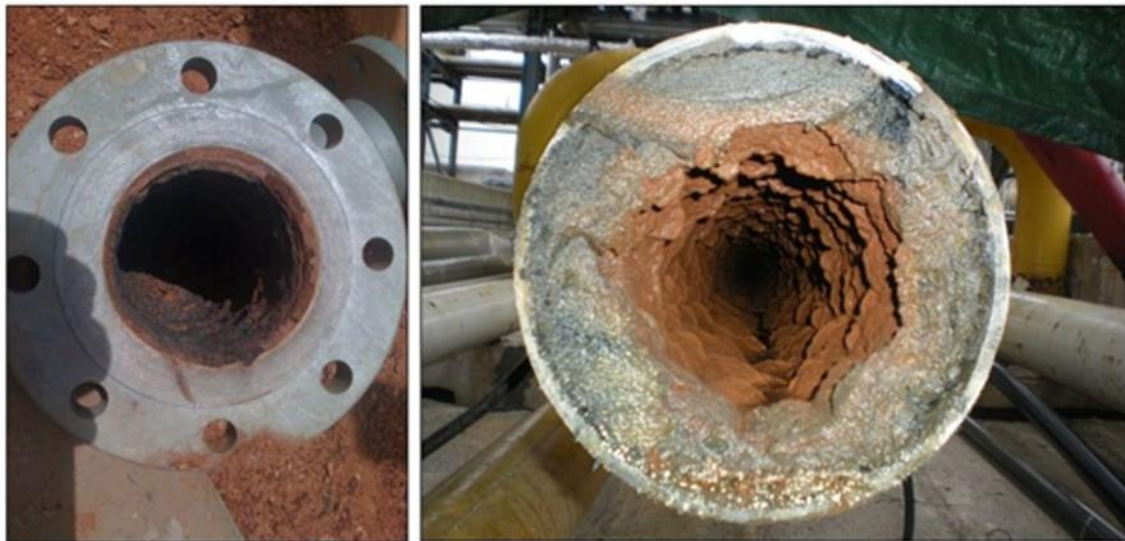
Figure 10. Iron and calcium contamination in pipework
