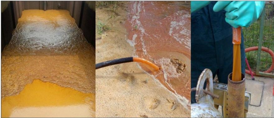
Figure 2. Discoloured water associated with pumping from wells suffering from iron deposits
