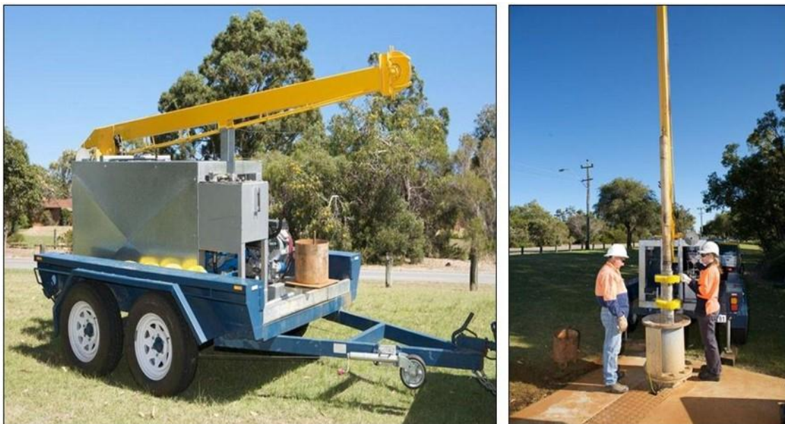
Figure 4. Well rehabilitation rig used in BoreSaver maintenance programmes
