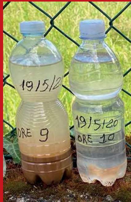
The sample bottle (left) shows how cloudy the water was and demonstrates the mud found in the borehole. The sample (right) was taken one hour later after the mechanical clean but before the chemical treatment
