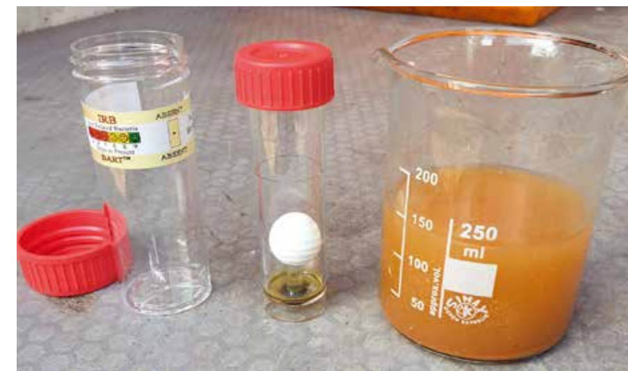
▲ Photo shows the test vial (centre) once it has been removed from the outer dispenser.
