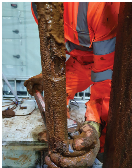
Photo shows typical iron bacteria residues on a pipe prior to treatment. © Drilcorp
